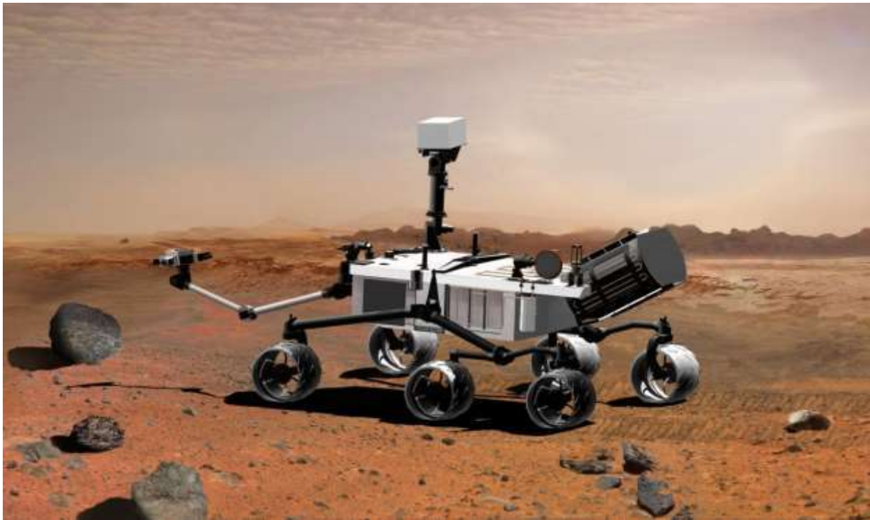
NASA’s Mars Rover is an autonomous robot that uses a 3D camera to map the planet’s surface. (iStock)
